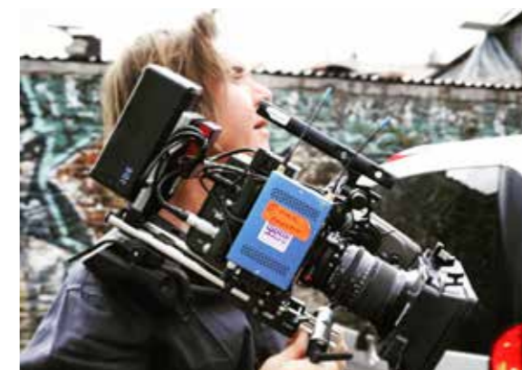
ALEXA Mini in documentary mode with 15mm bars, V-Lok battery, moose bars, SuperSpeed lens, LMB25 matte box, timecoded Lockit Box and audio receiver for guide track
