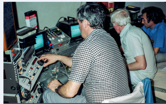
Mobile editing in a hotel room in Djibouti in 1986 – the Umatic edit suite weighed around 200kg and took a while to set up
