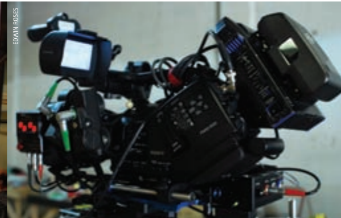
▲ The video was shot using the Sony EX3 (owned by the band) powered by an onboard Anton Bauer Dionic 90
