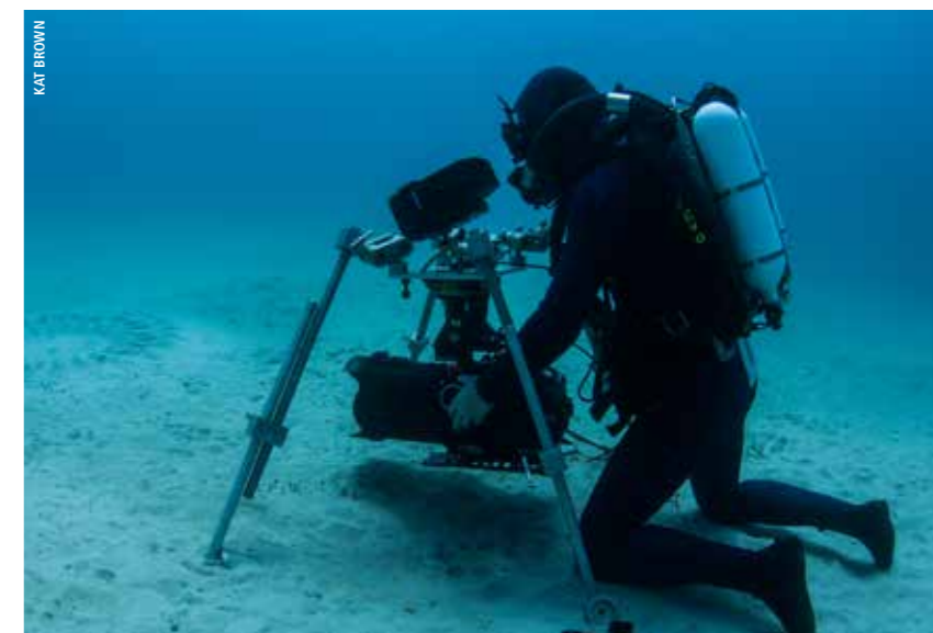
RED EPIC in a Gates housing, underslung on the custom-built quad mount
