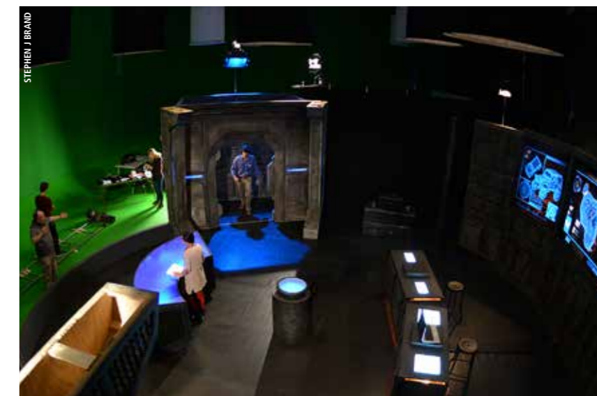
Figure 3 (top): The lighting would be high contrast with the futuristic technology (such as this central podium lit with a LitePanels Bicolour 1x1 panel and 'bright blue' gel) providing sources of light; Figure 4 (bottom): The set from the top shot showing the different areas
