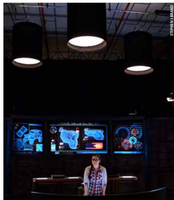
Figure 5: Filmgear 4.8kW space-lights overhead (skirted to control the spill)
