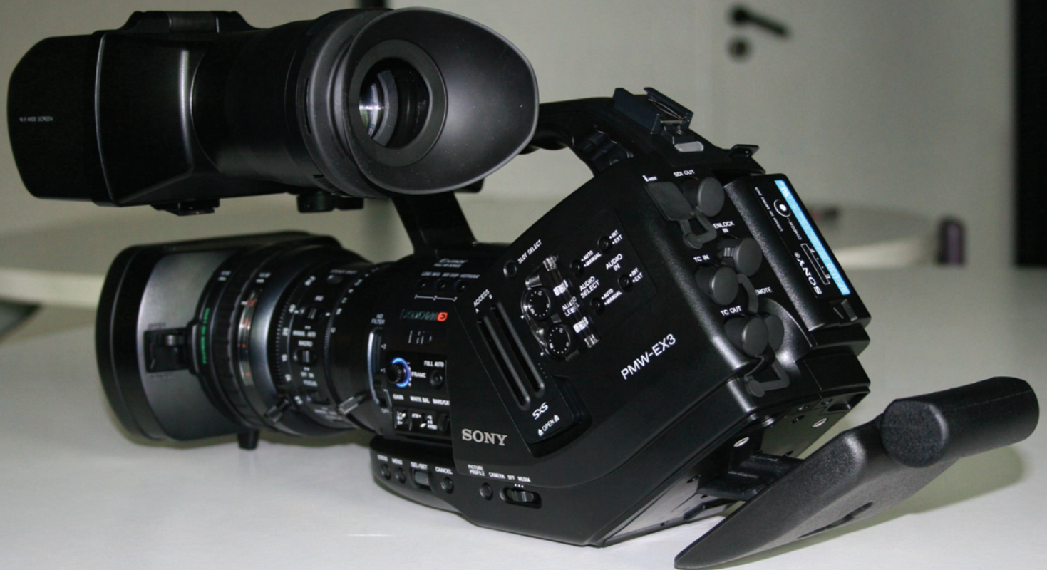
Wedge shape design with shoulder pad which slides in and out and will lock in position
