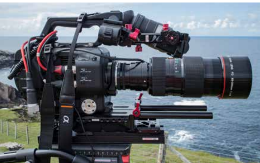
Vintage Canon FD 85–300mm lens converted by The Lens Doctor to EF mount and manual iris
