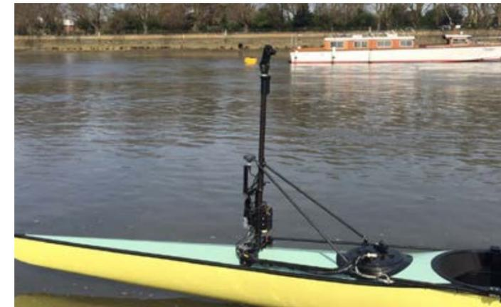
Camera Corps supply a specialist camera mounted on a mast to look down the length of each team boat, plus a camera looking up from the cox’s position
