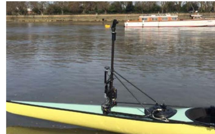
Camera Corps supply a specialist camera mounted on a mast to look down the length of each team boat, plus a camera looking up from the cox's position
