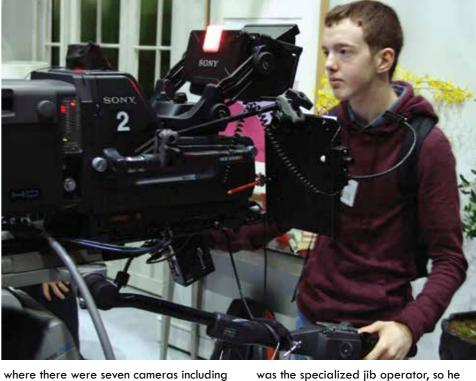
five pedestal cameras with box lenses and autocue, a handheld camera with a wideangle lens and a 9ft Jimmy Jib with a wideangle lens on the front. Before we got to work with the equipment we were greeted by Mel who works for the Vitec Group that supply pedestals and camera support systems to the industry. He gave us a talk on the health and safety aspects of gassing a pedestal and what to be aware of when operating the pedestal such as the speed of the pedestal rising and falling.
