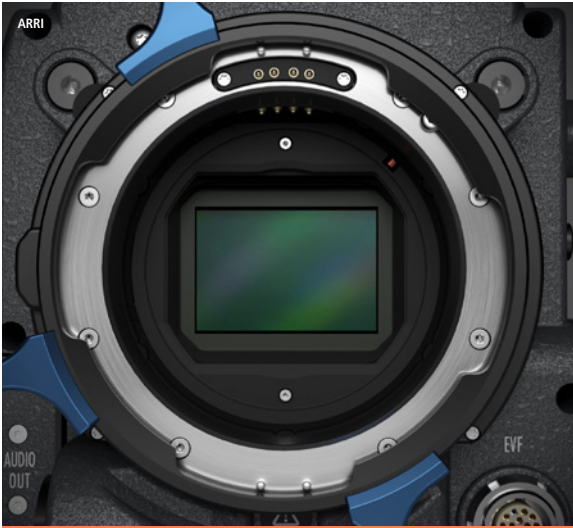
Above: The ALEV III (A2X) CMOS 4.5K sensor of the ARRI ALEXA LF Left: DIT Eduardo Eguia offers some insight into how HDE enhanced his workflow on Disney's The Mandalorian Inset: The ALEXA Mini LF with Compact Drive
