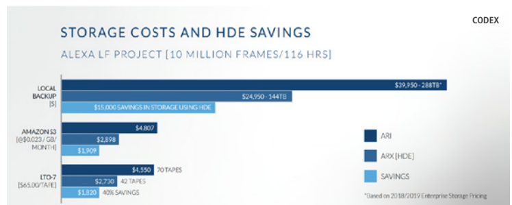
An illustration of the relative costs incurred when storing ARRIRAW files compared to the equivalent HDE encoded files, which demonstrates the savings that can be made
