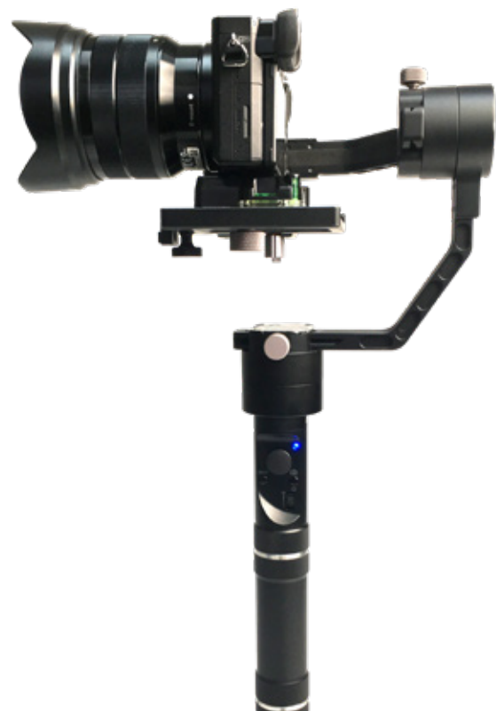
The Zhiyun Crane V2 can carry up to 1.8kg, but what if your camera combo is too light? This Sony a6300 and 10–18mm lens only weigh 670g, which is great news for your wrists but can be difficult to balance. Adding a quick-release plate raises the CoG sufficiently.
