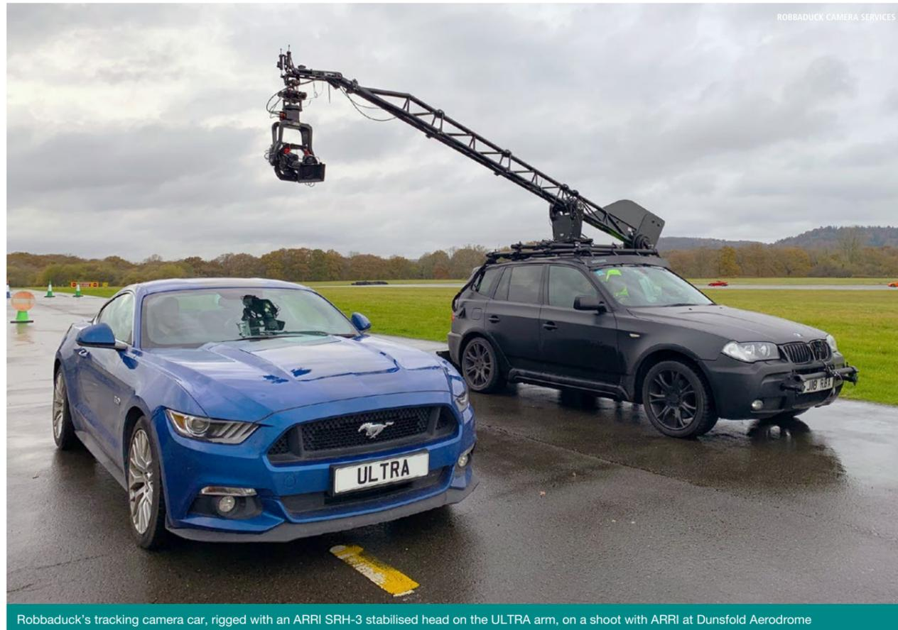
Robbaduck's tracking camera car, rigged with an ARRI SRH-3 stabilised head on the ULTRA arm, on a shoot with ARRI at Dunsfold Aerodrome
