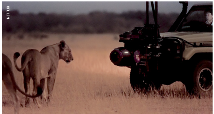
The car-mounted Shotover F1 gimbal allows immersive action footage – on the move, at lion eye level
