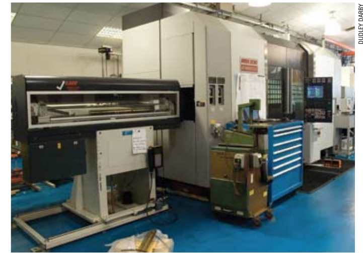
▲ Numerically controlled milling machine producing small parts from brass rod
