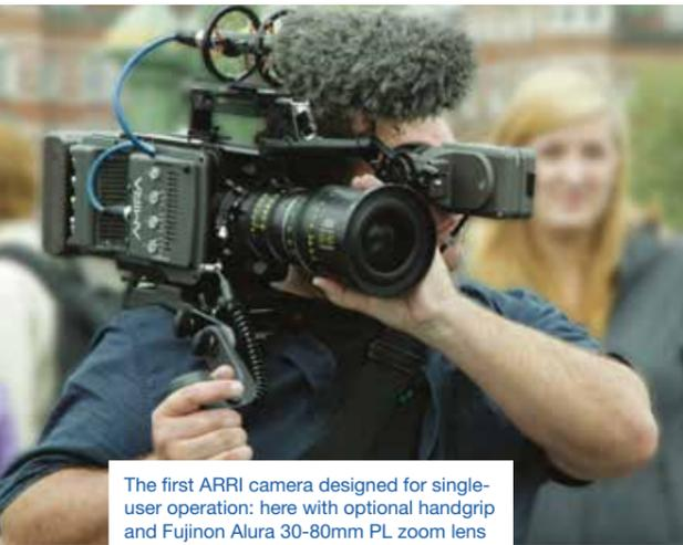
The first ARRI camera designed for single-user operation: here with optional handgrip and Fujinon Alura 30-80mm PL zoom lens
