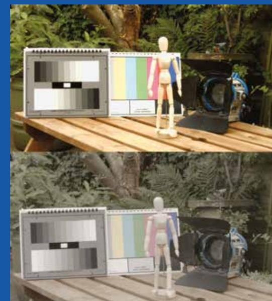
**Top:** A Rec.709 image, exposed to average the scene and retain some shadow detail, but at the expense of clipped highlights.
